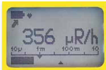
Approaching a source Alarm thresholds - not yet exceeded Trend arrow indicates increasing radiation level
